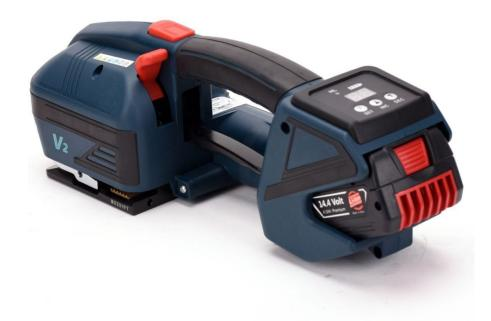
product name:BATTERY POWERED PLASTIC STRAPPING band width:13-16mm band thickness:0/4-1/2mm strain force:3200n battery:14/4v-4000mah-batteryx2 charging time:1/5h capacity:250-350 tapes when fully charged dimension:380x130x130mm tension speed:100-200mm/s weight:3/1kg
