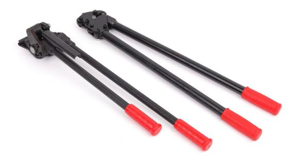
product name:MANUAL STEEL STRAPPING 32mm <u>TENSIONER</u> band width:16-32mm band thickness:0/8-1/2mm sealing type:with buckle weight:3/8kg <u>SEALER</u> band width:32mm band thickness:0/6-1/2mm locking type:double tooth handle Lenght:650mm weight:3/5kg
