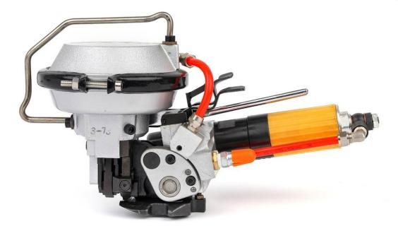
product name:PNEUMATIC COMBINATION STEEL STRAPPING 16mm band width:16-19mm band thickness:0/5-0/8mm function:tighten+lock+cut air pressure:0/42-0/63mpa strain force:4500n dimension:350x170x160mm tension speed:60mm/min weight:4/2kg
