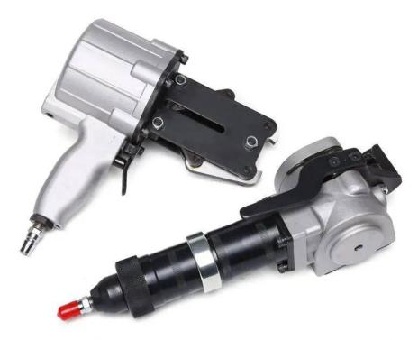
product name:PNEUMATIC TENSIONER AND SEALER STEEL STRAPPING 32mm band width:32mm band thickness:0/8-1/2mm function:tighten+lock+cut air pressure:0/49-0/63mpa strain force:8500n dimension:TENSIONER 320x100x200mm SEALER 200x200x100mm tension speed (with no load):5100mm/min weight:clamping machine 4,8kg+locking machine 3/2kg=8kg
