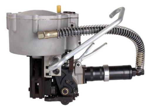
product name:PNEUMATIC COMBINATION STEEL STRAPPING 32mm band width:32mm band thickness:0/8-1/2mm function:tighten+lock+cut air pressure:0/35-0/63mpa strain force:9800n dimension:430x280x410mm tension speed:530mm/min weight:15kg
